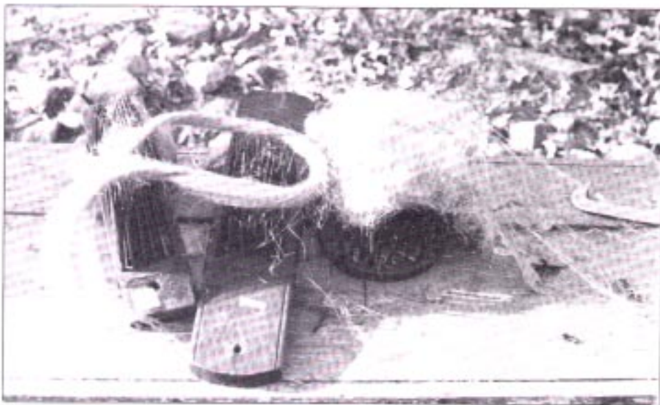
Three sizes of hackles, wicked-looking tools. Start with the teeth farthest apart to comb the flax. End with the finer tool. What remains of the flax bundle in my hand is the LINE. The TOW collects between the teeth, right.
