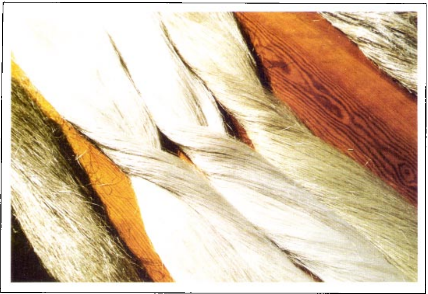
12. Hackled flax: 1. to r. :ground retted line, 2 stricks of water-retted line, and 1 strick of early-harvested water-retted line
