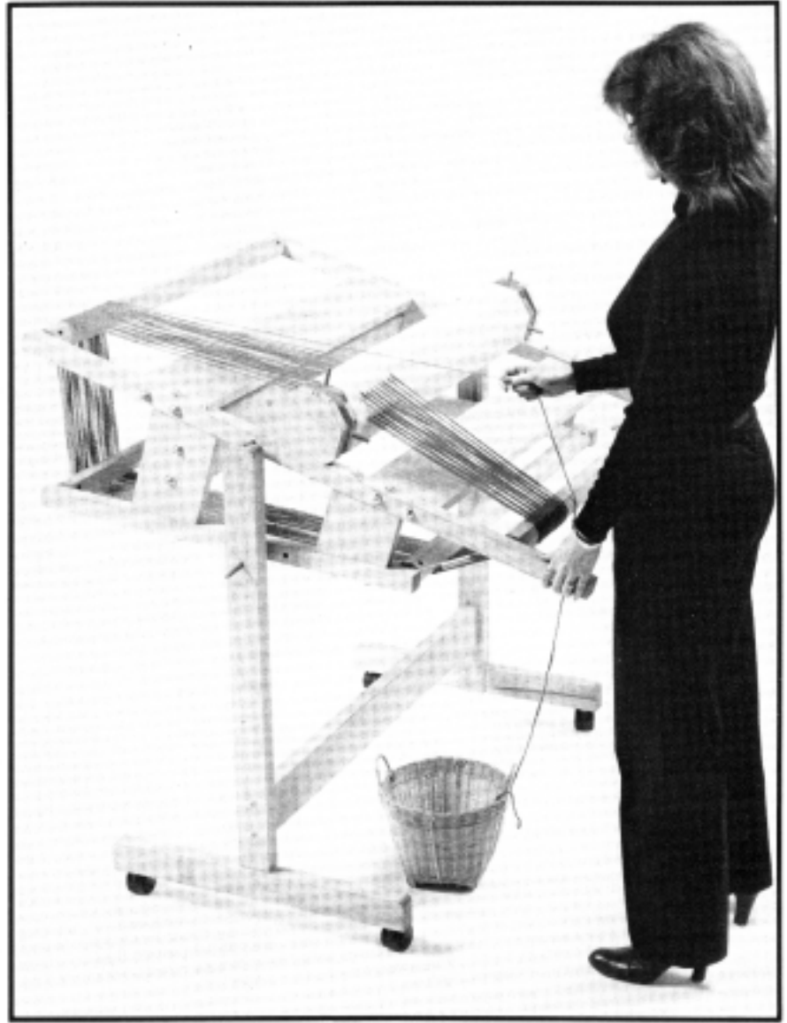
FIGURE 9. Warping the MasterWeaver loom
