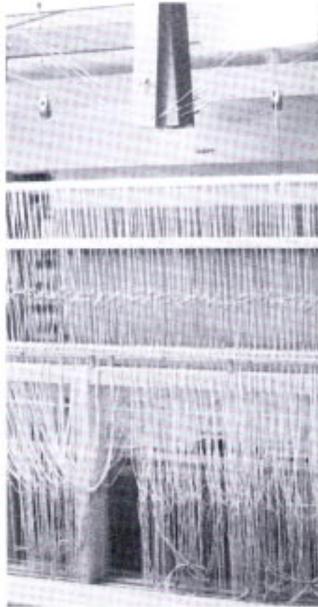
3. Shaft-switcher mounted on a counter-march loom with vertical jacks. The doups are ready to be threaded.
