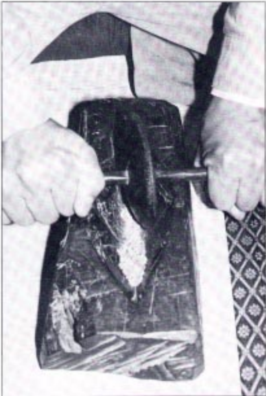
This tool is from Miyazaki Prefecture in the southeastern section of Kyushu Island. It was used to grind dye materials. The substance was placed in the trough and pulverized by turning the wheel over it. According to the owner, this grinder is now obsolete.
