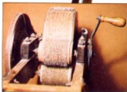
"Spin-well" drum carder with 3 drums. (1) Detail of 3-drum arrangement. (1)
