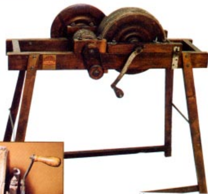
"Spin-well" drum carder with 3 drums. (1) Detail of 3-drum arrangement. (1)
