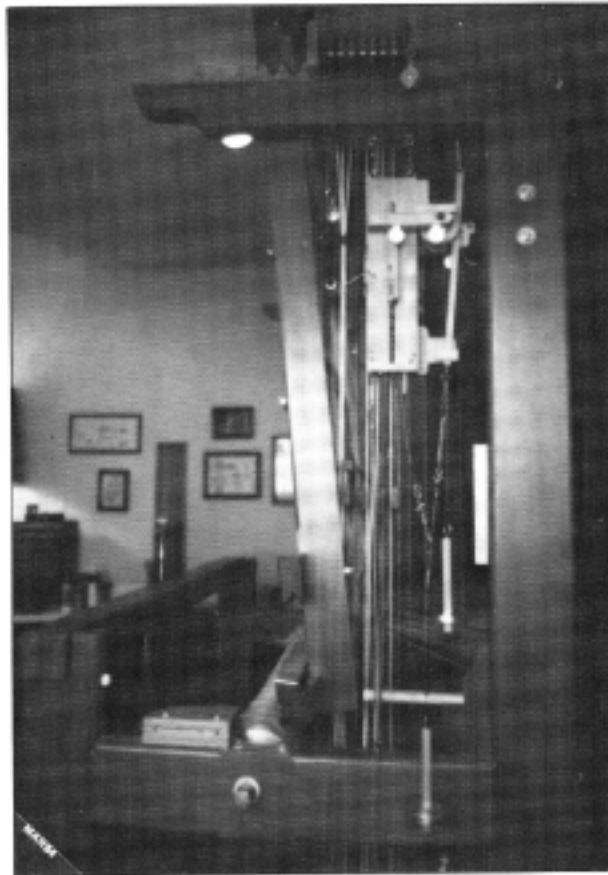
Doublejack on Mr. Koepp's loom, breast beam on the left. Loom side is 5 inches wide, the beater is 3 inches wide. Note the counterweights.
