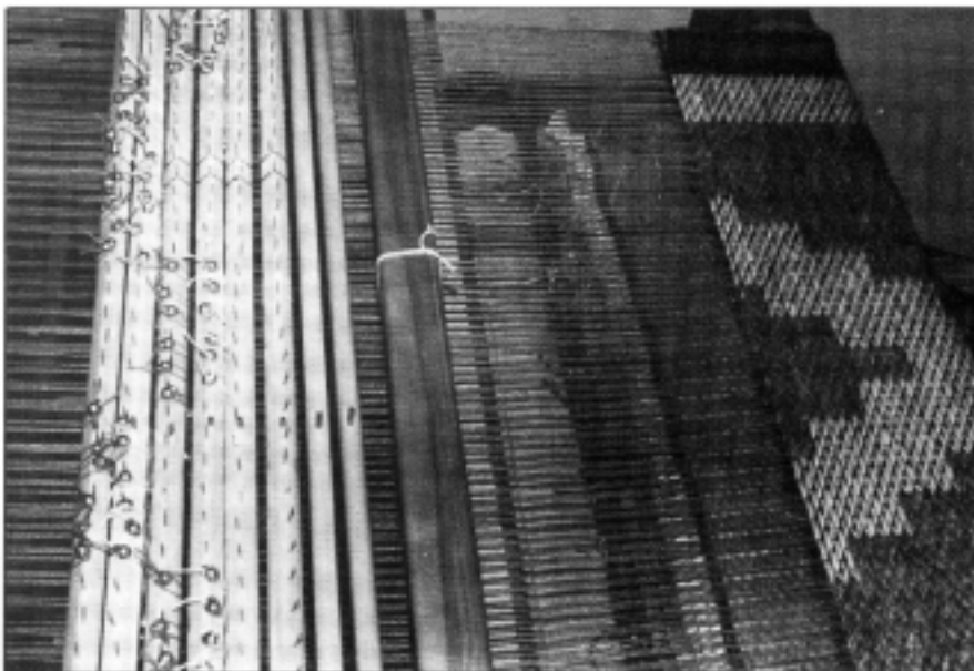
View from above showing shaft-switching racks.
