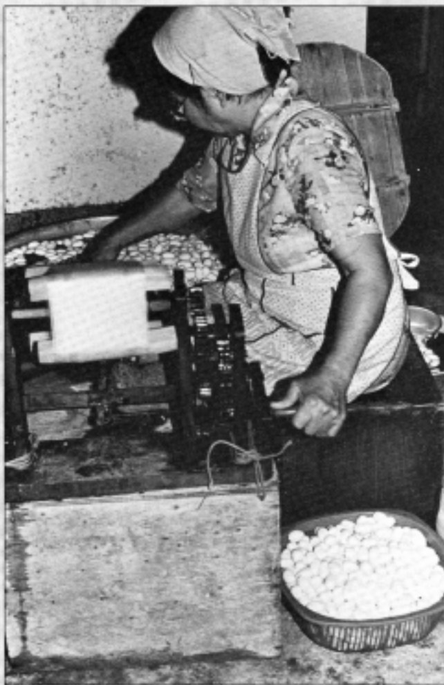
Above, strands of silk are reeled onto a wooden spool mounted on a winding apparatus.
