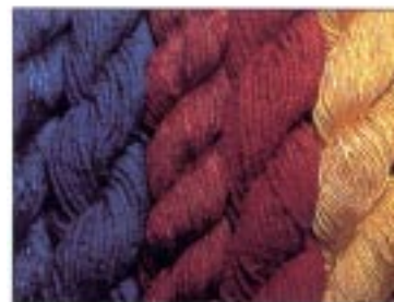
The difference in luster between a noil yarn and a high quality spun Bombyx.
