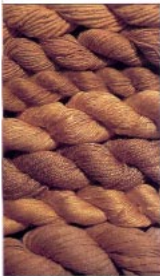
A variety of wild silks and Bombyx showing how each has accepted a yellow dye (Lanaset).
