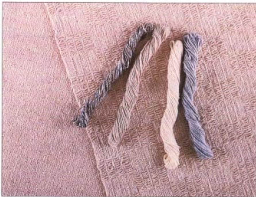
4/2 cotton samples shown on place mats woven by June Ann Fish of Albuquerque using 4/2 burnt cotton sett at 20 e.p.i.
