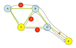
Figure 1: Path exploration triggered by a fail-down event.
