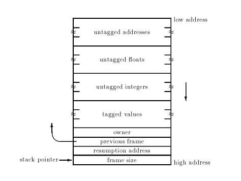
Figure 1. Structure of a Stack Frame in jc
