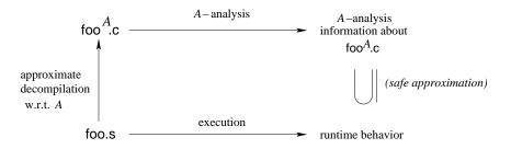
Figure 4. Using approximate decompilation for program analysis
